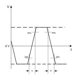
Figure 1.1. Differential Waveform Definition
