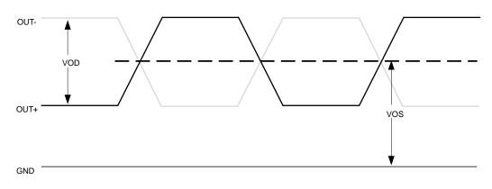
Figure 1.2. Differential Output – Single-Ended View
