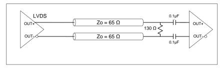
Figure 3.3. LVDS Single AC Termination at the Load
