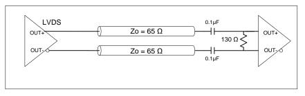
Figure 3.2. LVDS Single AC Termination at the Load
