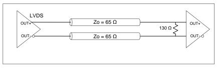
Figure 3.1. LVDS Single AC Termination at the Load
