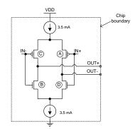
Figure 2.1. LVDS Driver Output Structure
