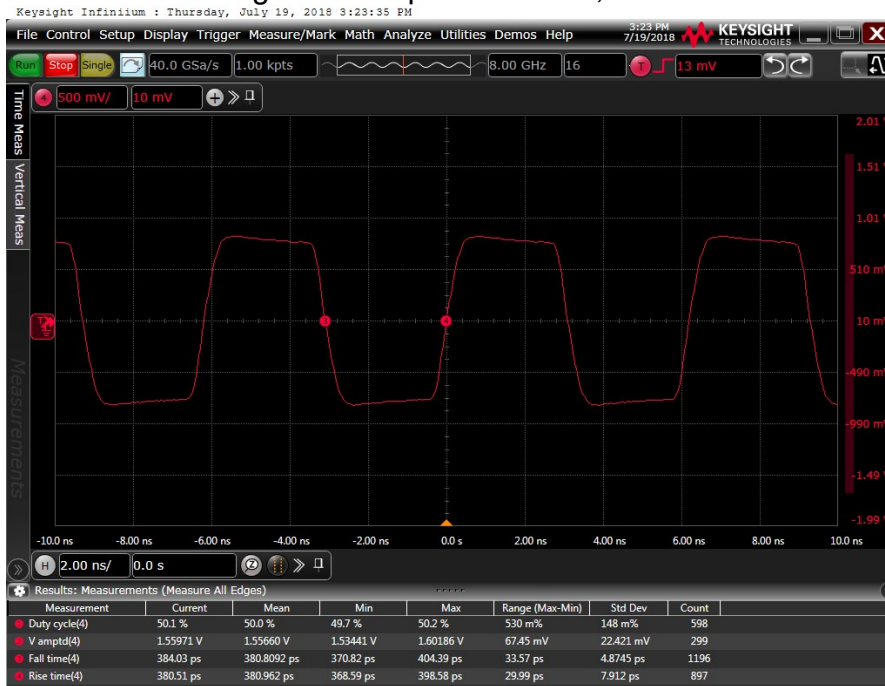
Figure 3: Output waveform, 3.3 V
