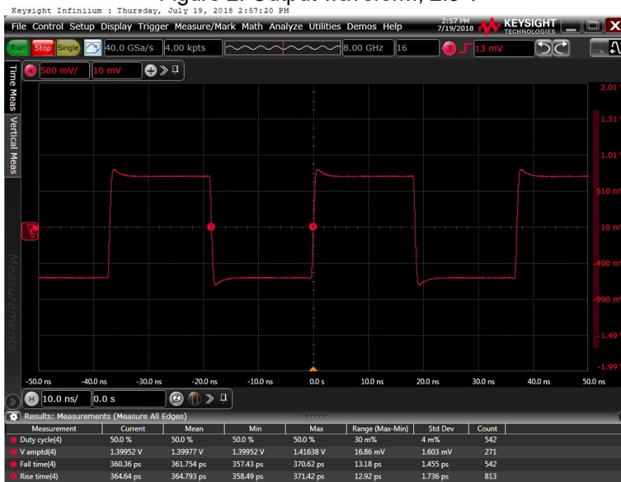
Figure 3: Output waveform, 3.3 V
