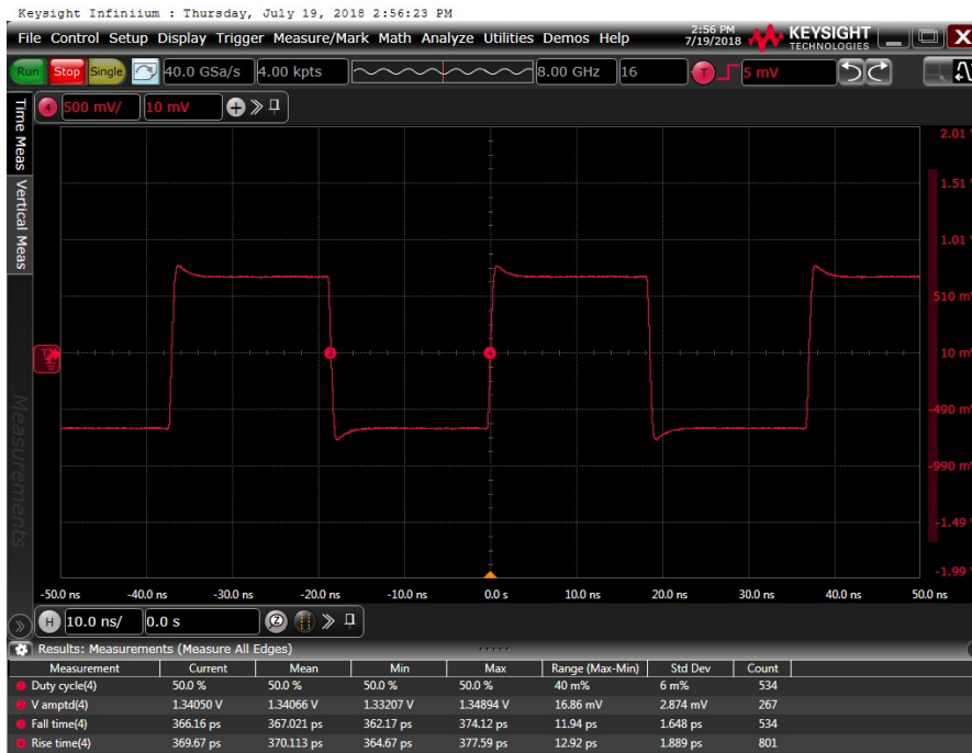
Figure 2: Output waveform, 2.5 V
