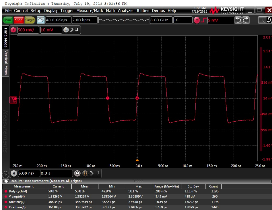
Figure 2: Output waveform, 2.5 V
