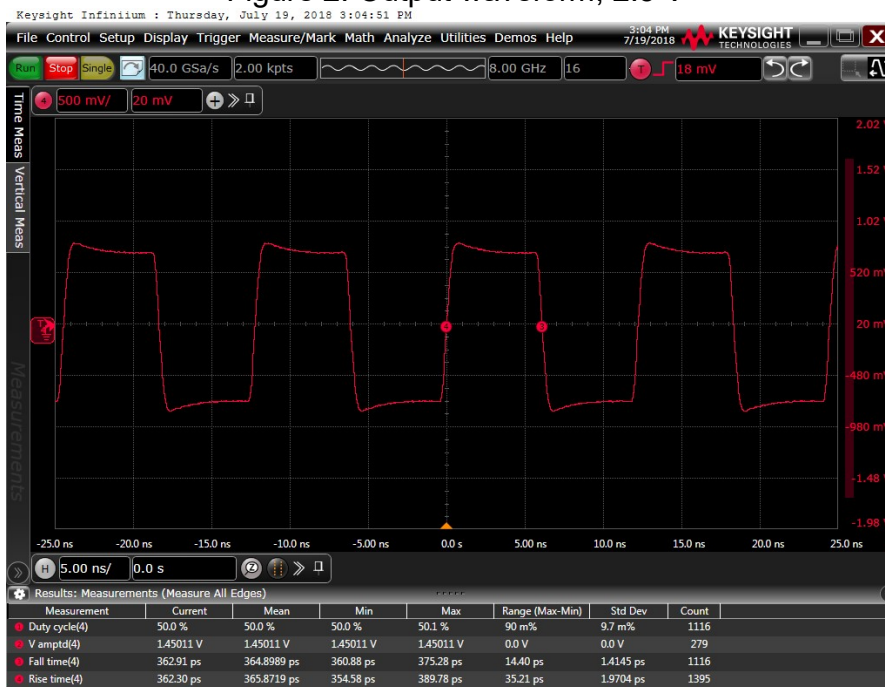
Figure 3: Output waveform, 3.3 V
