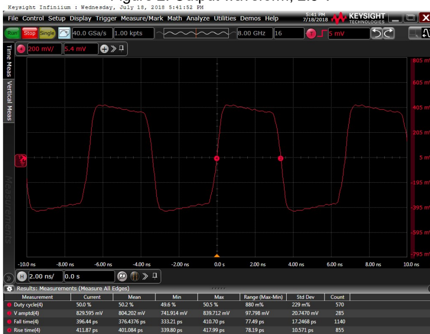
Figure 3: Output waveform, 3.3 V
