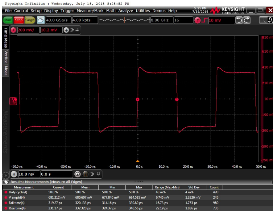
Figure 2: Output waveform, 2.5 V
