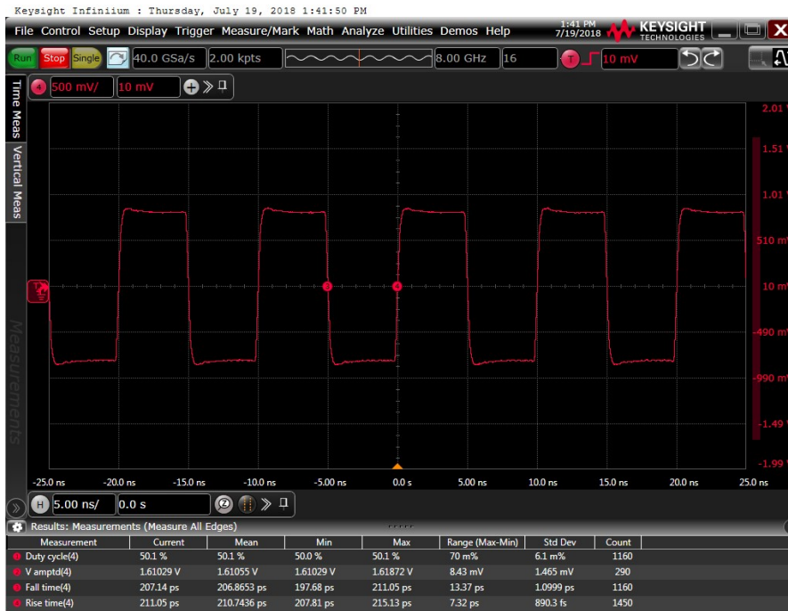
Figure 2: Output waveform, 2.5 V
