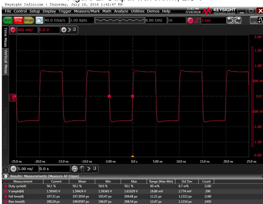
Figure 3: Output waveform, 3.3 V
