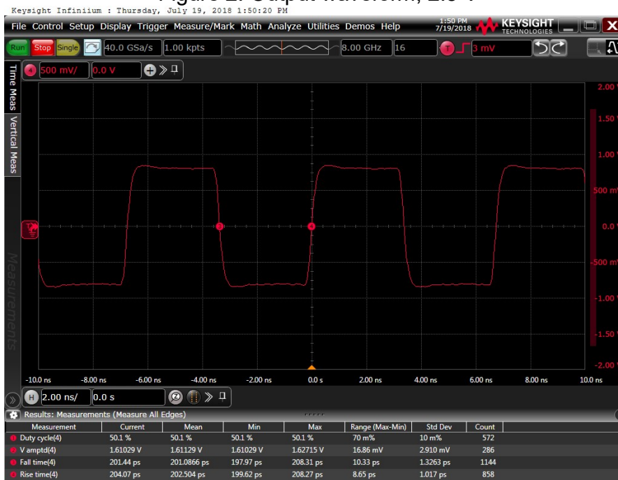
Figure 3: Output waveform, 3.3 V
