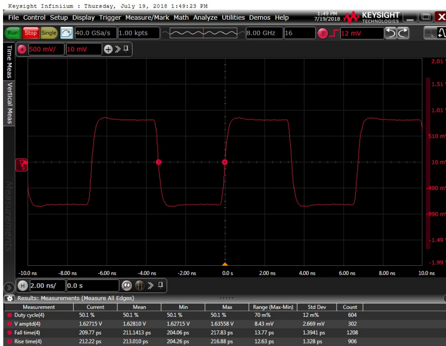
Figure 2: Output waveform, 2.5 V
