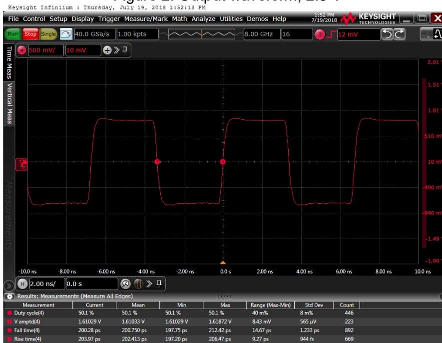
Figure 3: Output waveform, 3.3 V
