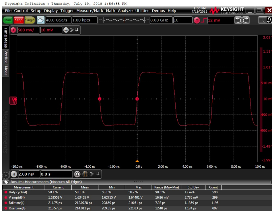
Figure 2: Output waveform, 2.5 V
