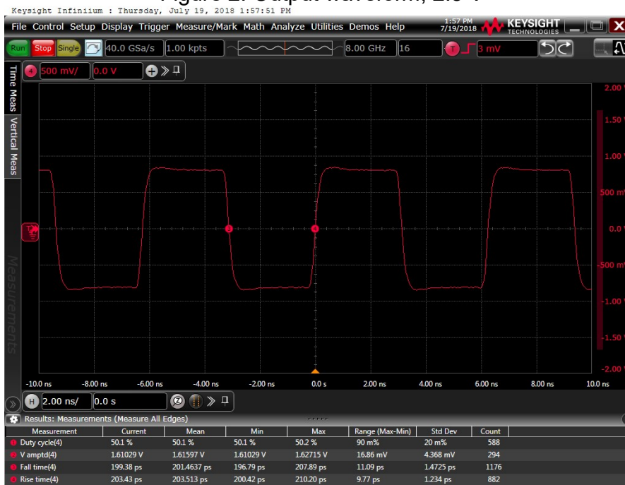
Figure 3: Output waveform, 3.3 V
