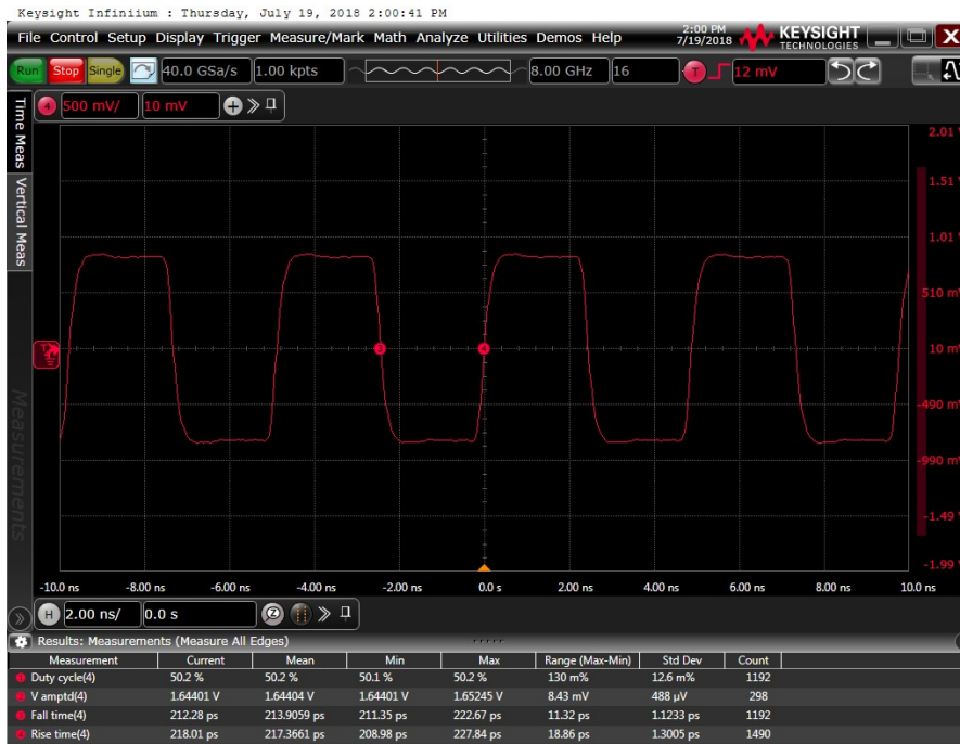
Figure 2: Output waveform, 2.5 V
