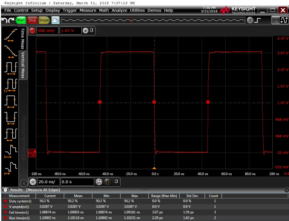
Figure 17: Output waveform, 3.0 V
