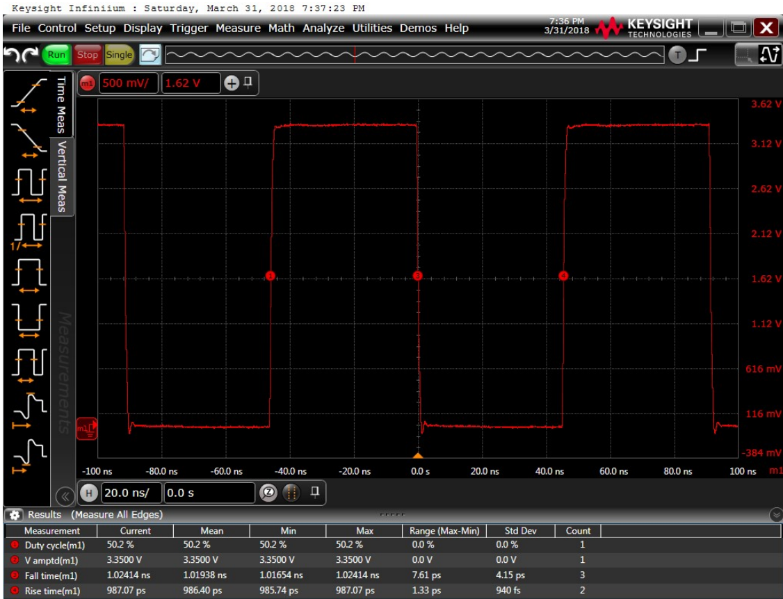
Figure 18: Output waveform, 3.3 V
