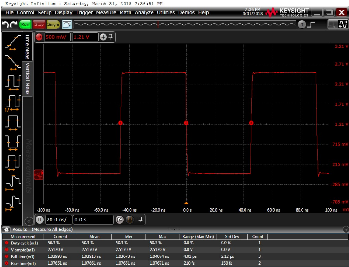
Figure 15: Output waveform, 2.5 V
