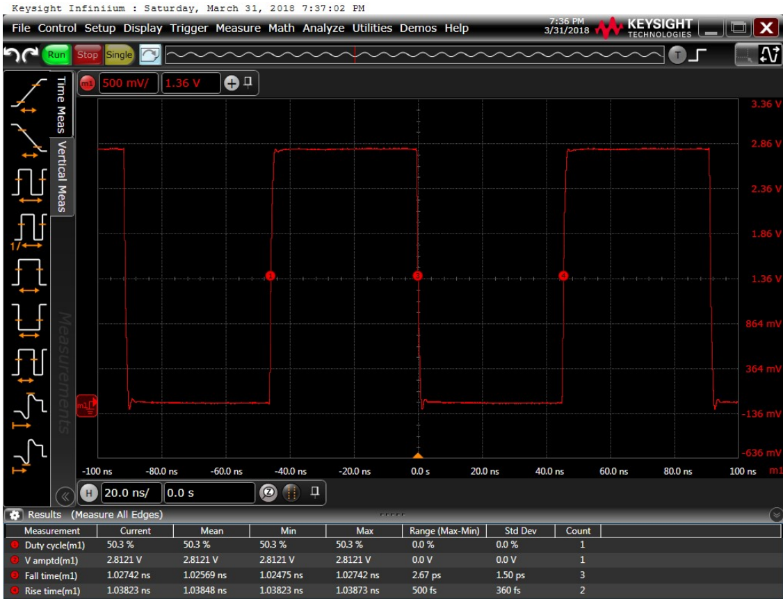
Figure 16: Output waveform, 2.8 V
