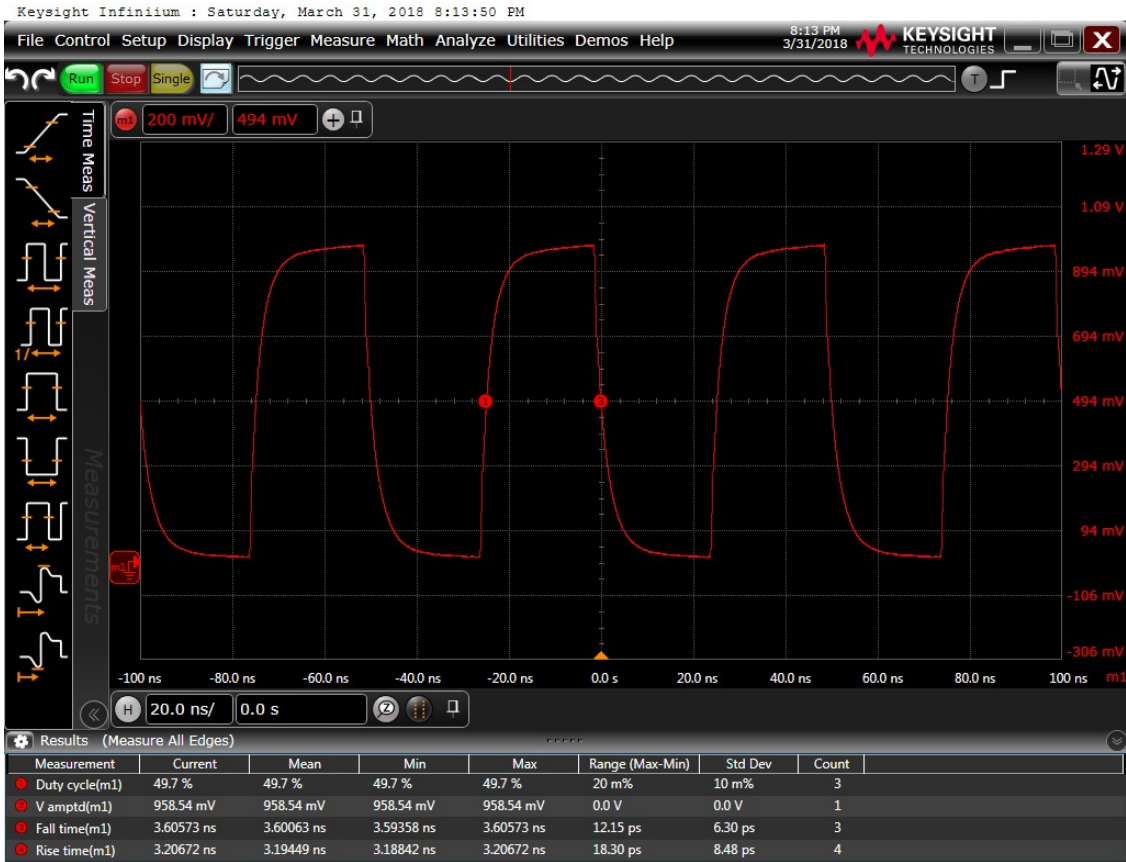
Figure 17: Output waveform, 3.0 V
