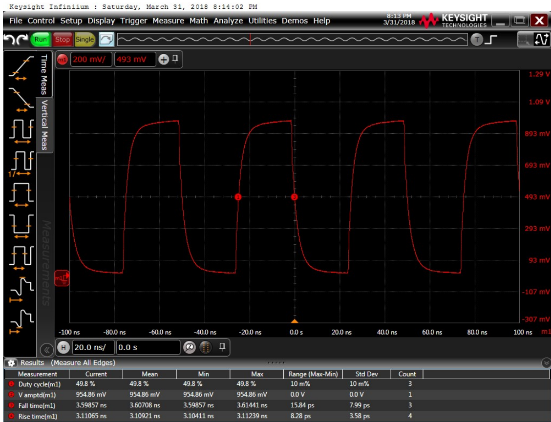
Figure 18: Output waveform, 3.3 V
