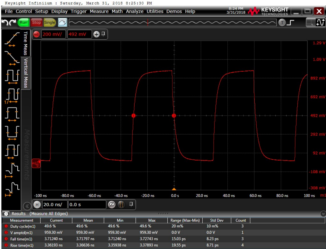
Figure 15: Output waveform, 2.5 V
