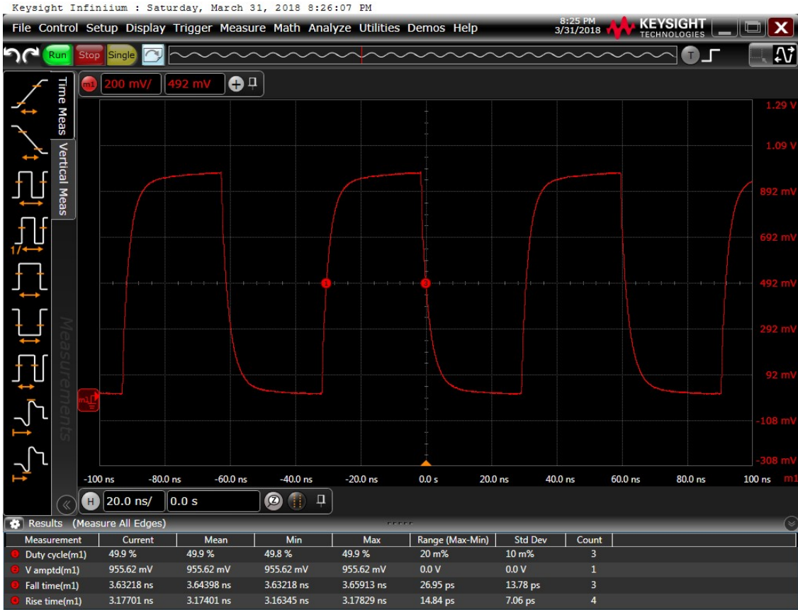
Figure 18: Output waveform, 3.3 V
