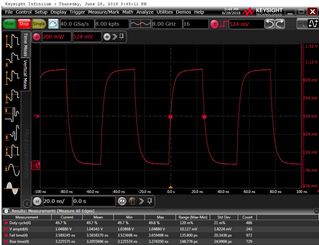
Figure 18: Output waveform, 3.3 V
