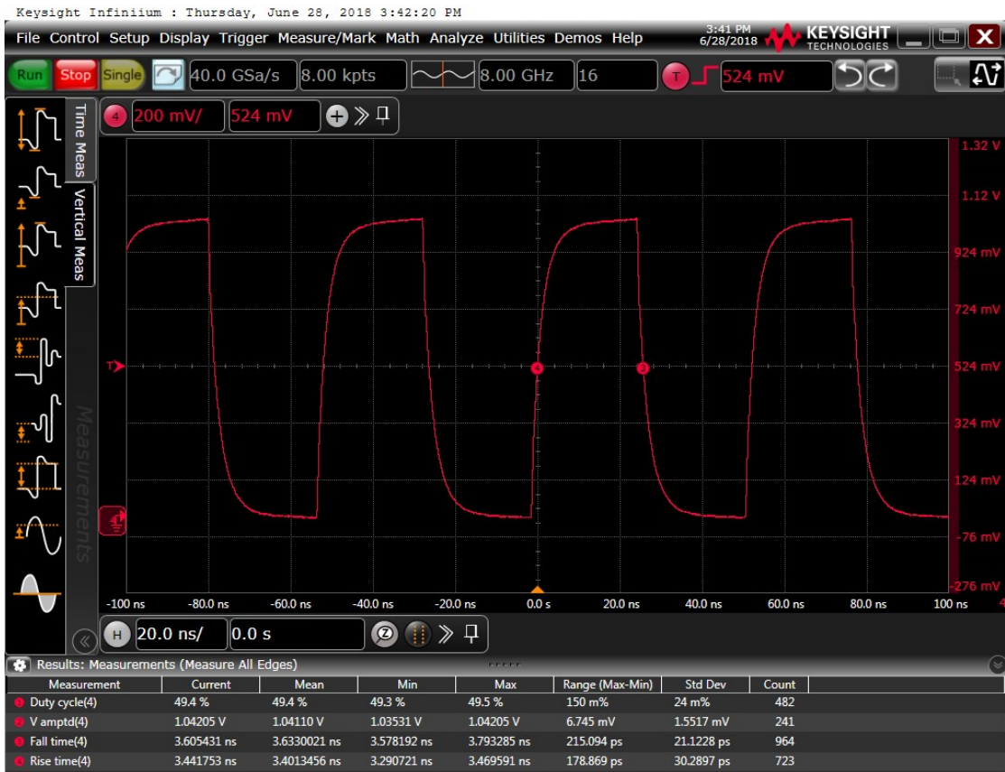
Figure 15: Output waveform, 2.5 V
