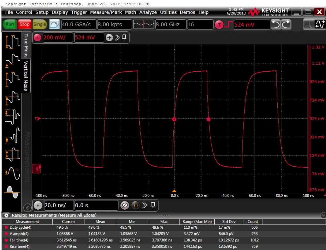
Figure 16: Output waveform, 2.8 V
