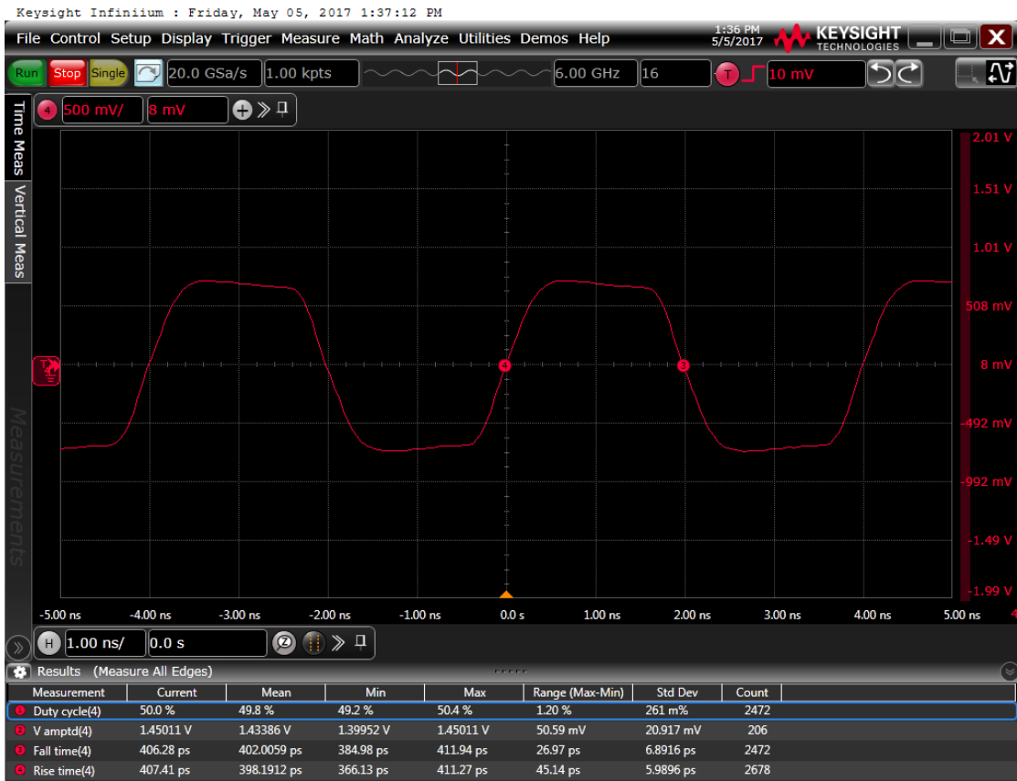
Figure 6: Output waveform, 2.5 V
