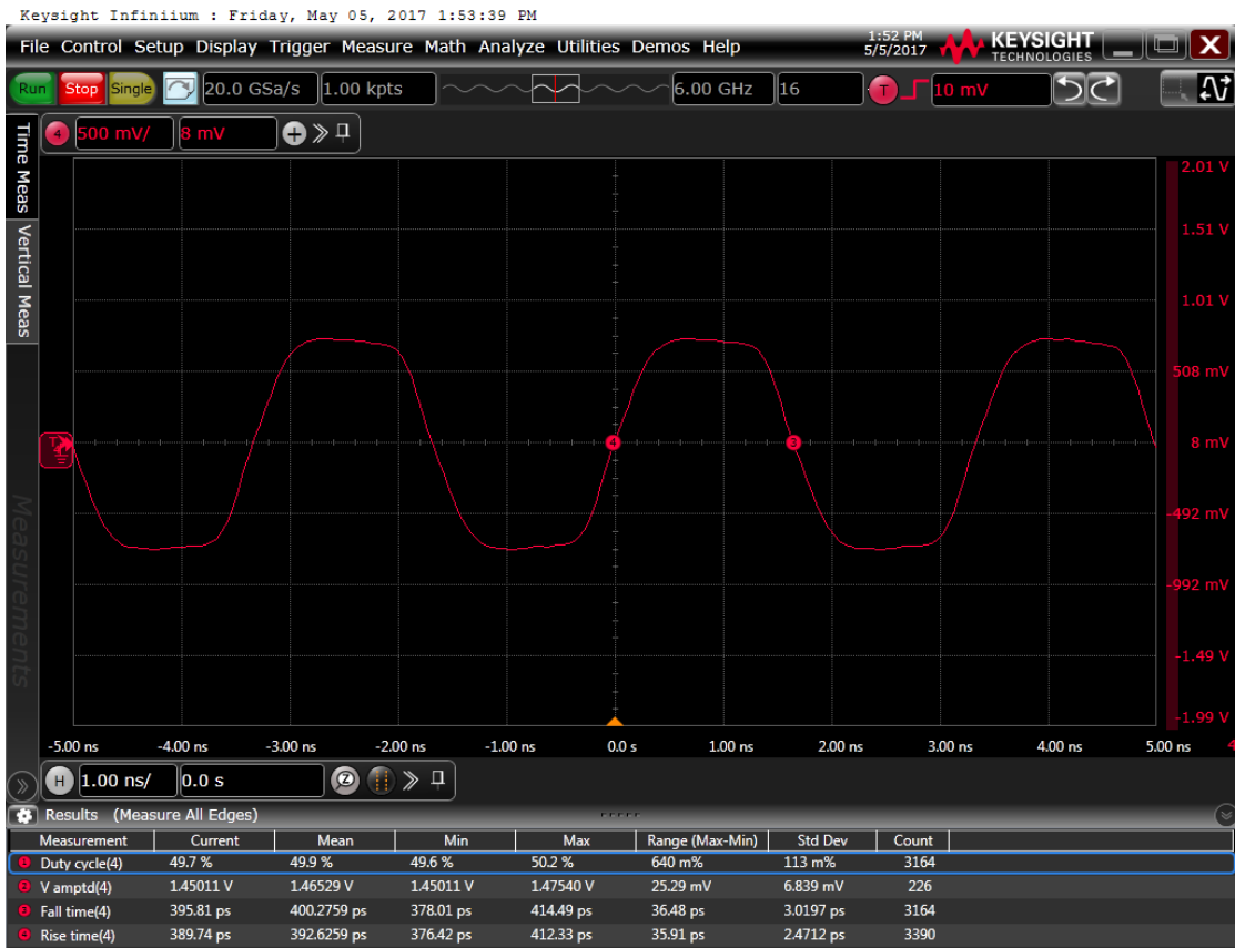
Figure 6: Output waveform, 2.5 V
