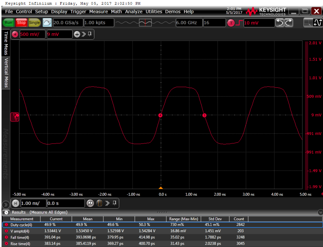
Figure 7: Output waveform, 3.3 V
