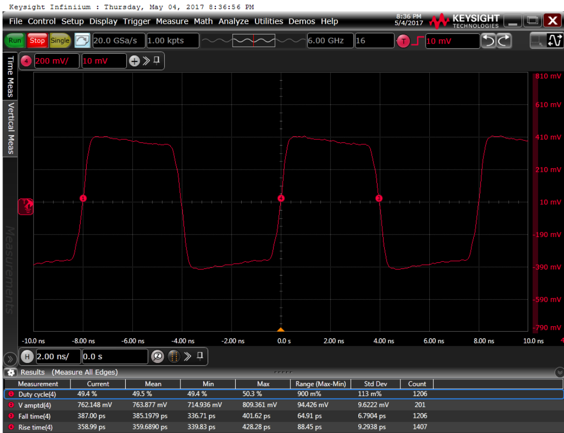
Figure 7: Output waveform, 3.3 V
