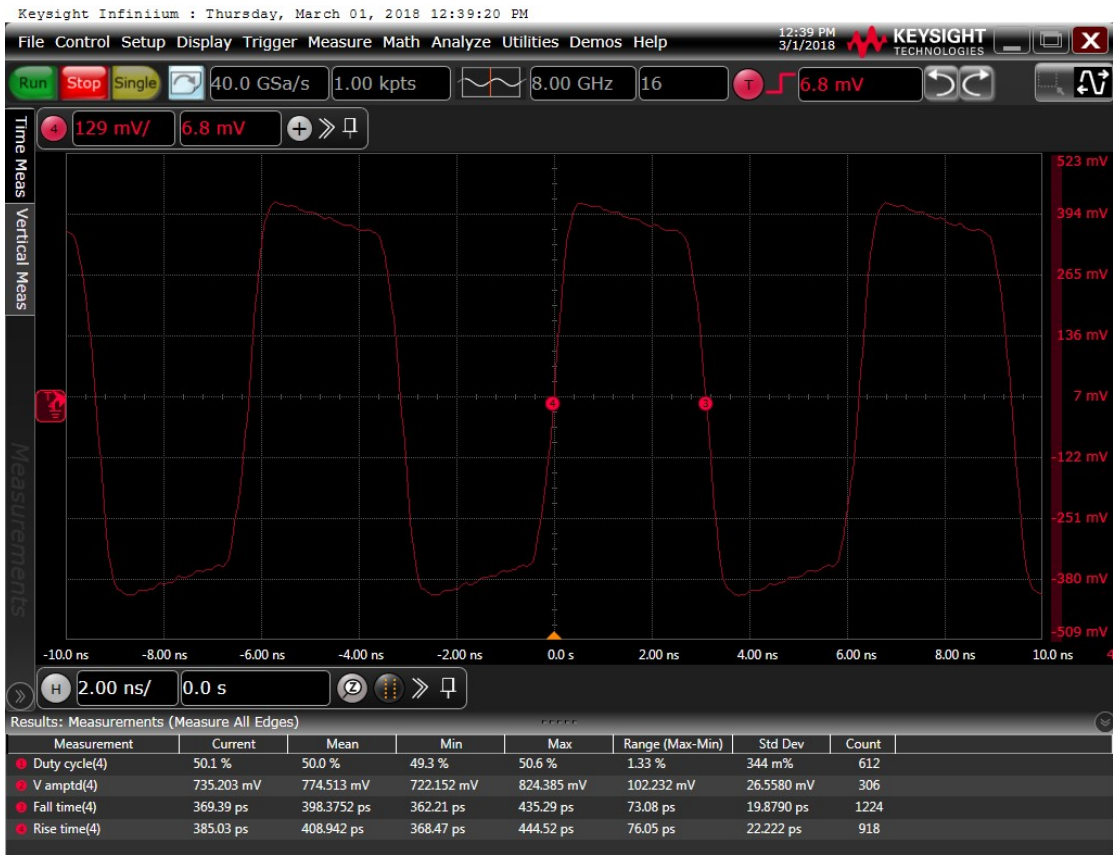
Figure 7: Output waveform, 3.3 V
