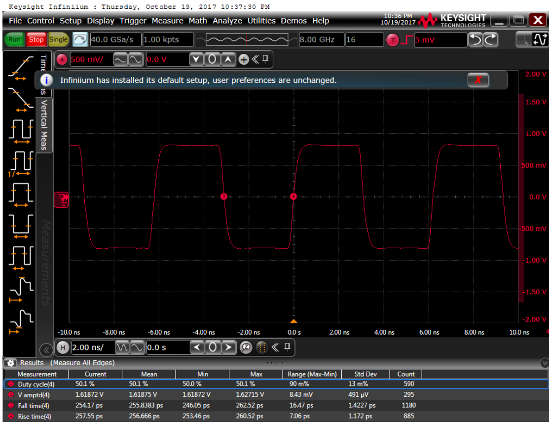
Figure 6: Output waveform, 2.5 V
