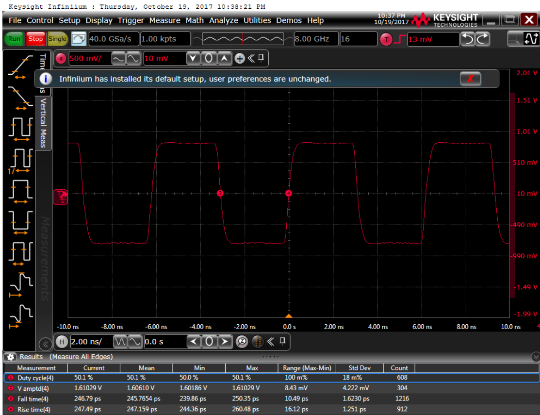
Figure 7: Output waveform, 3.3 V
