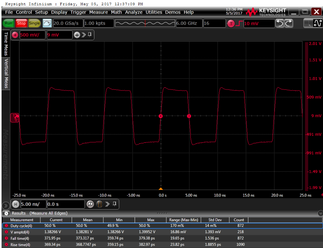
Figure 6: Output waveform, 2.5 V
