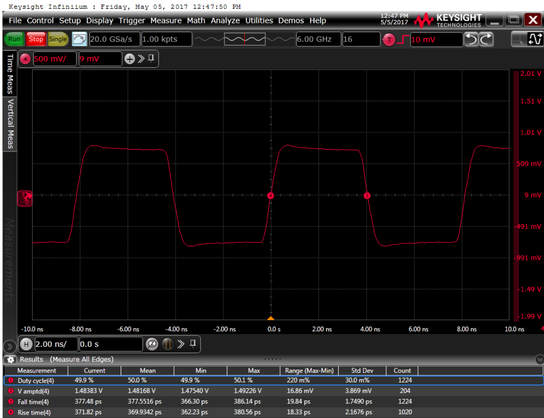
Figure 7: Output waveform, 3.3 V
