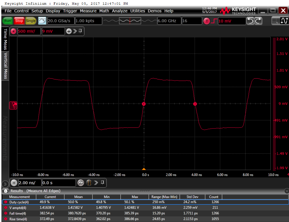
Figure 6: Output waveform, 2.5 V
