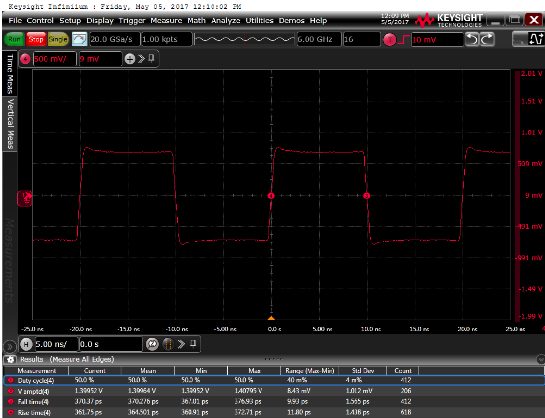
Figure 7: Output waveform, 3.3 V
