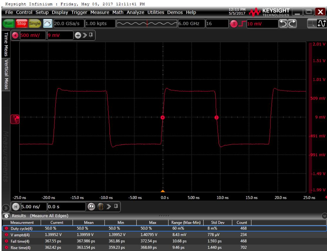
Figure 7: Output waveform, 3.3 V
