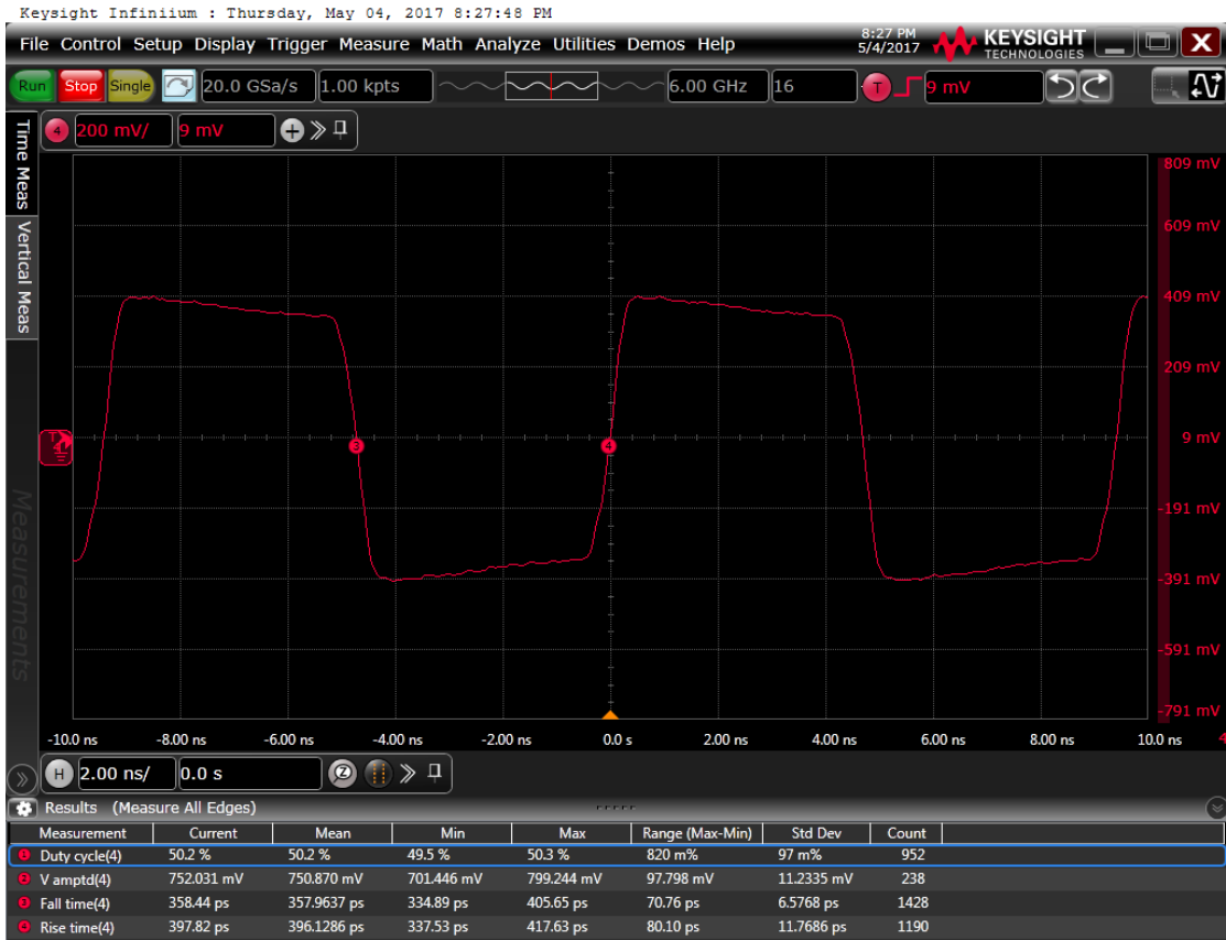
Figure 6: Output waveform, 2.5 V
