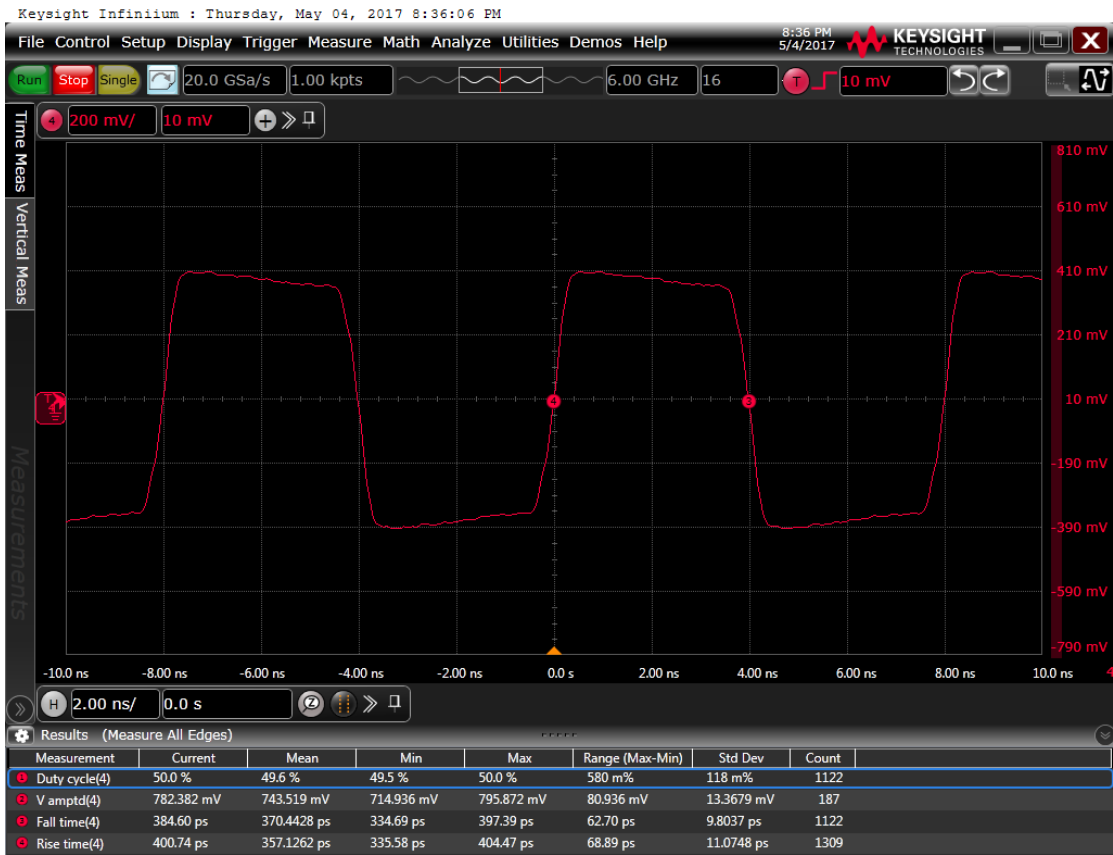
Figure 6: Output waveform, 2.5 V
