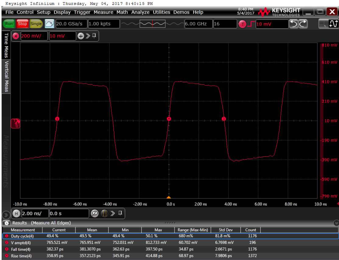
Figure 7: Output waveform, 3.3 V
