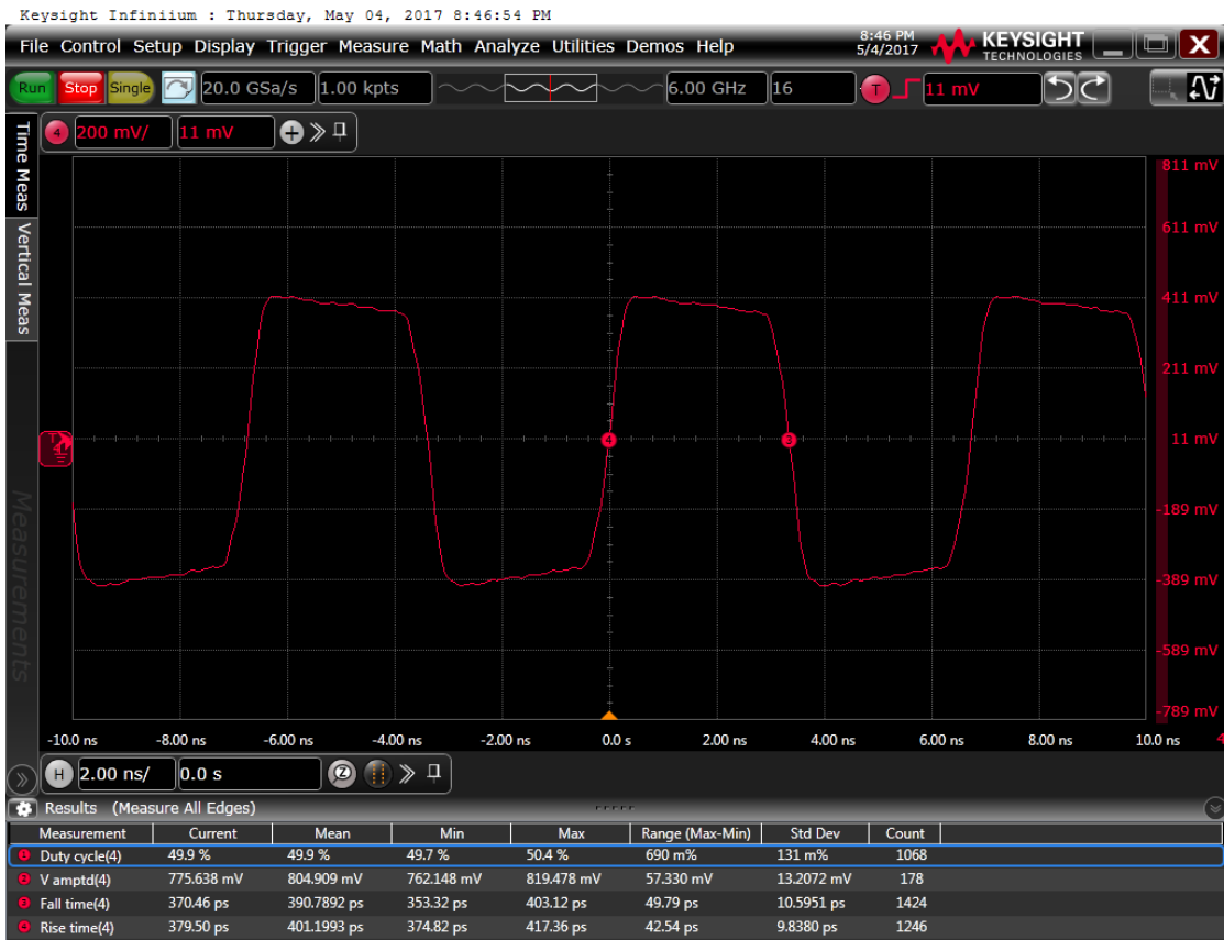
Figure 7: Output waveform, 3.3 V
