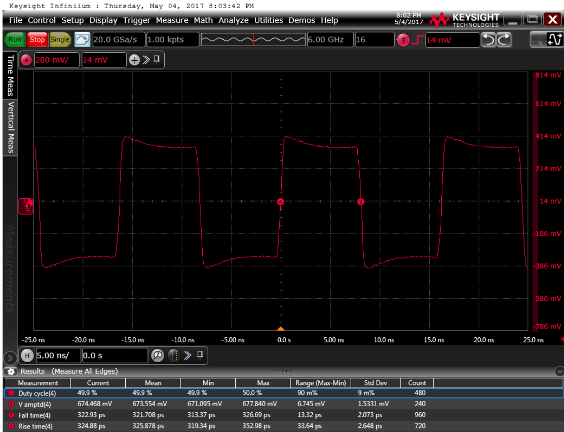
Figure 7: Output waveform, 3.3 V
