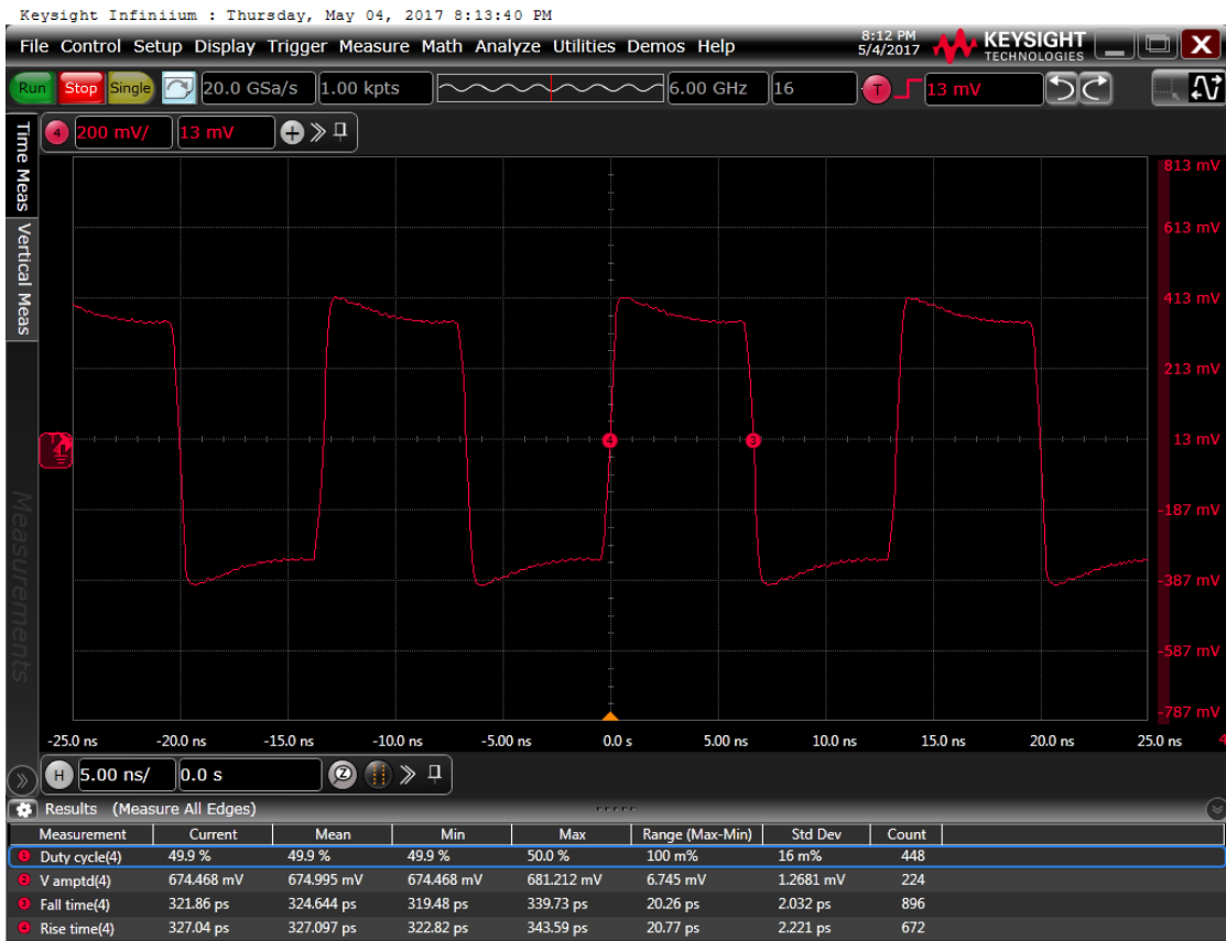
Figure 7: Output waveform, 3.3 V
