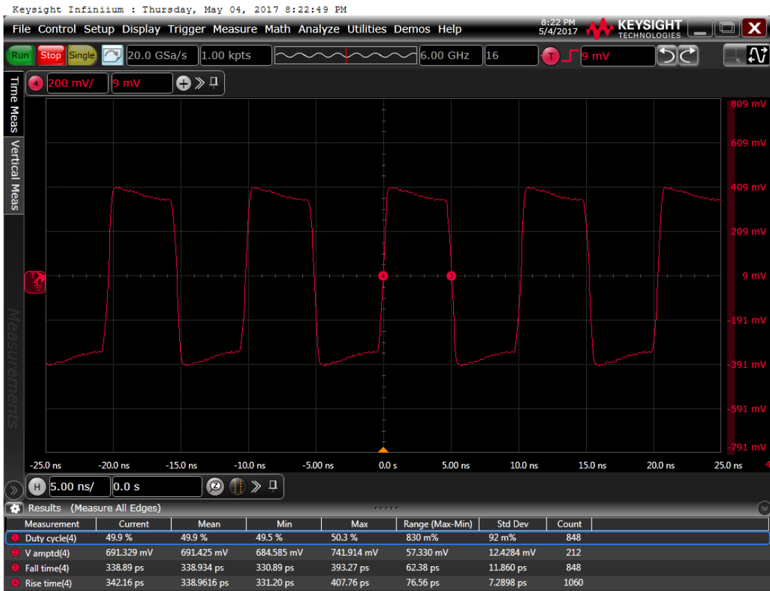
Figure 6: Output waveform, 2.5 V
