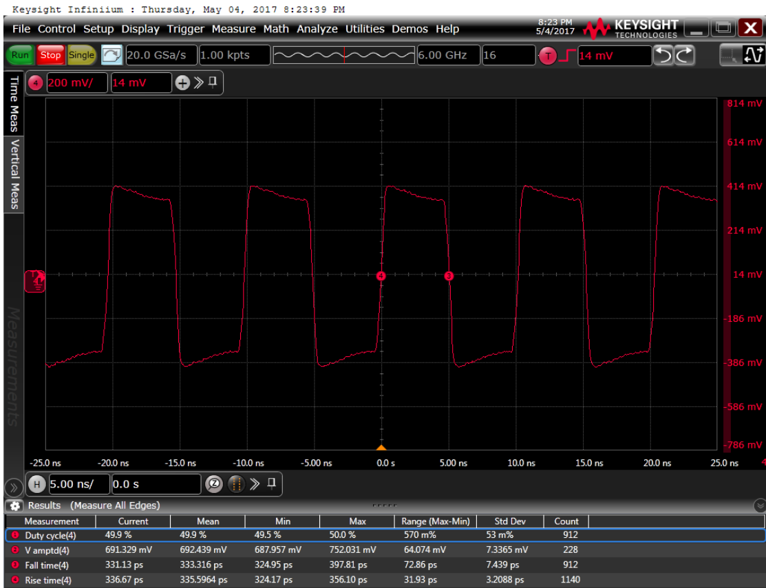
Figure 7: Output waveform, 3.3 V
