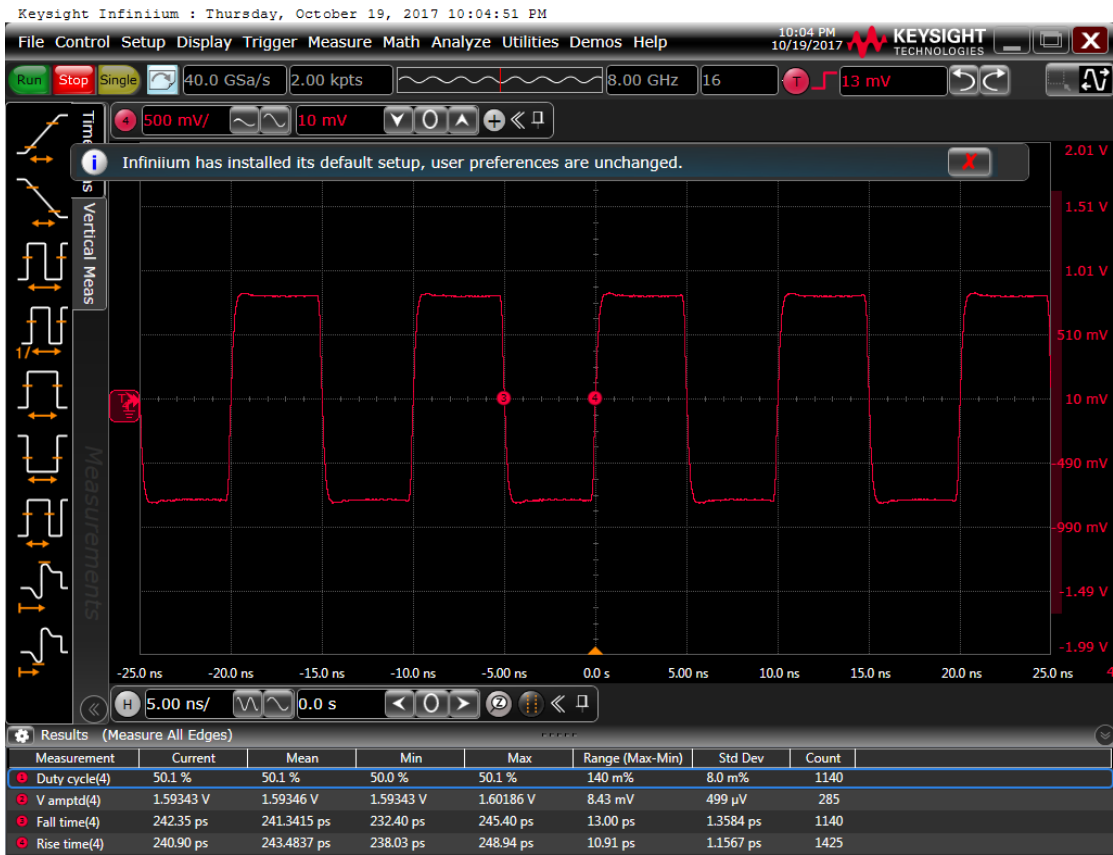
Figure 7: Output waveform, 3.3 V
