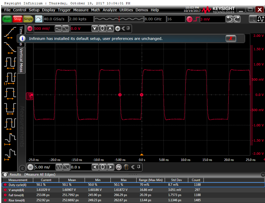
Figure 6: Output waveform, 2.5 V
