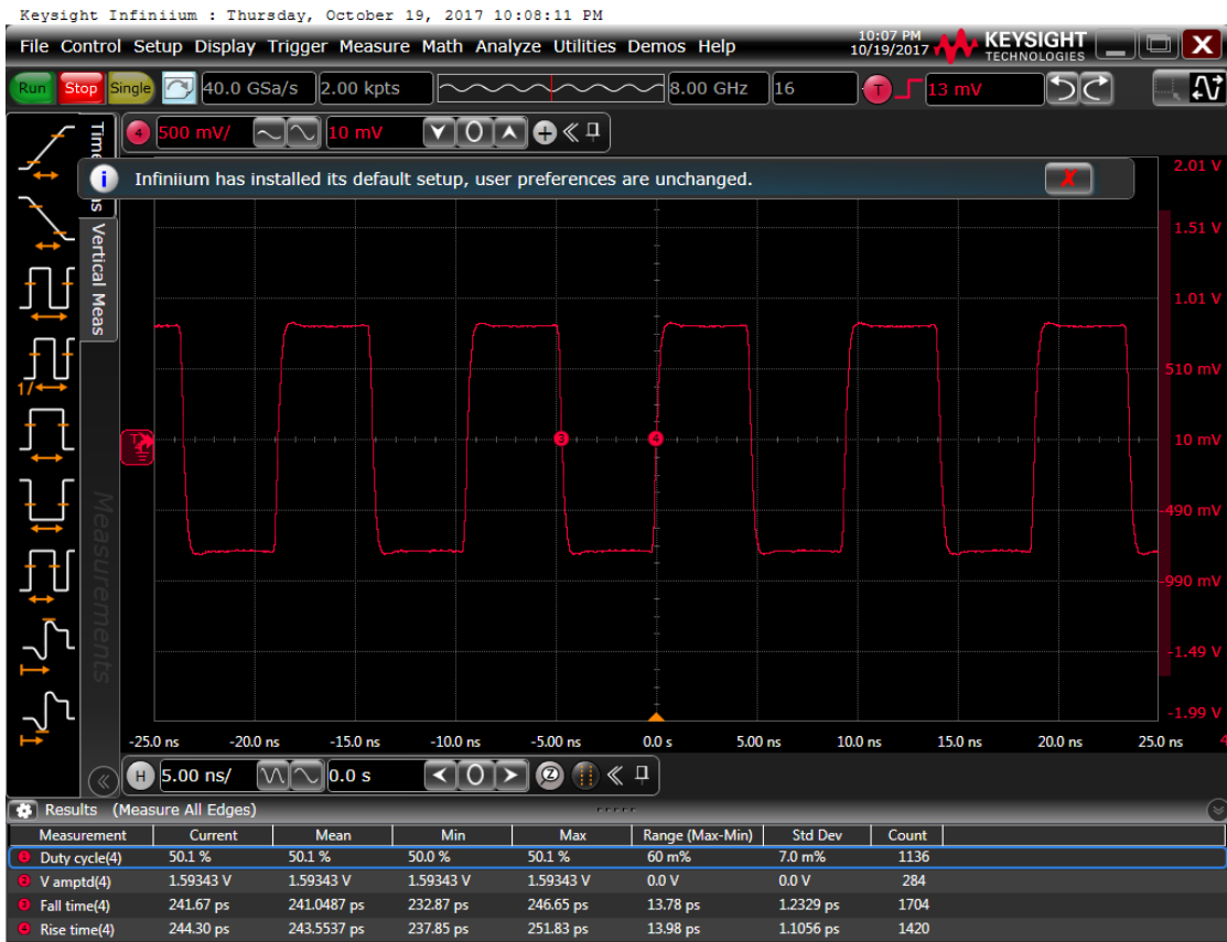
Figure 7: Output waveform, 3.3 V
