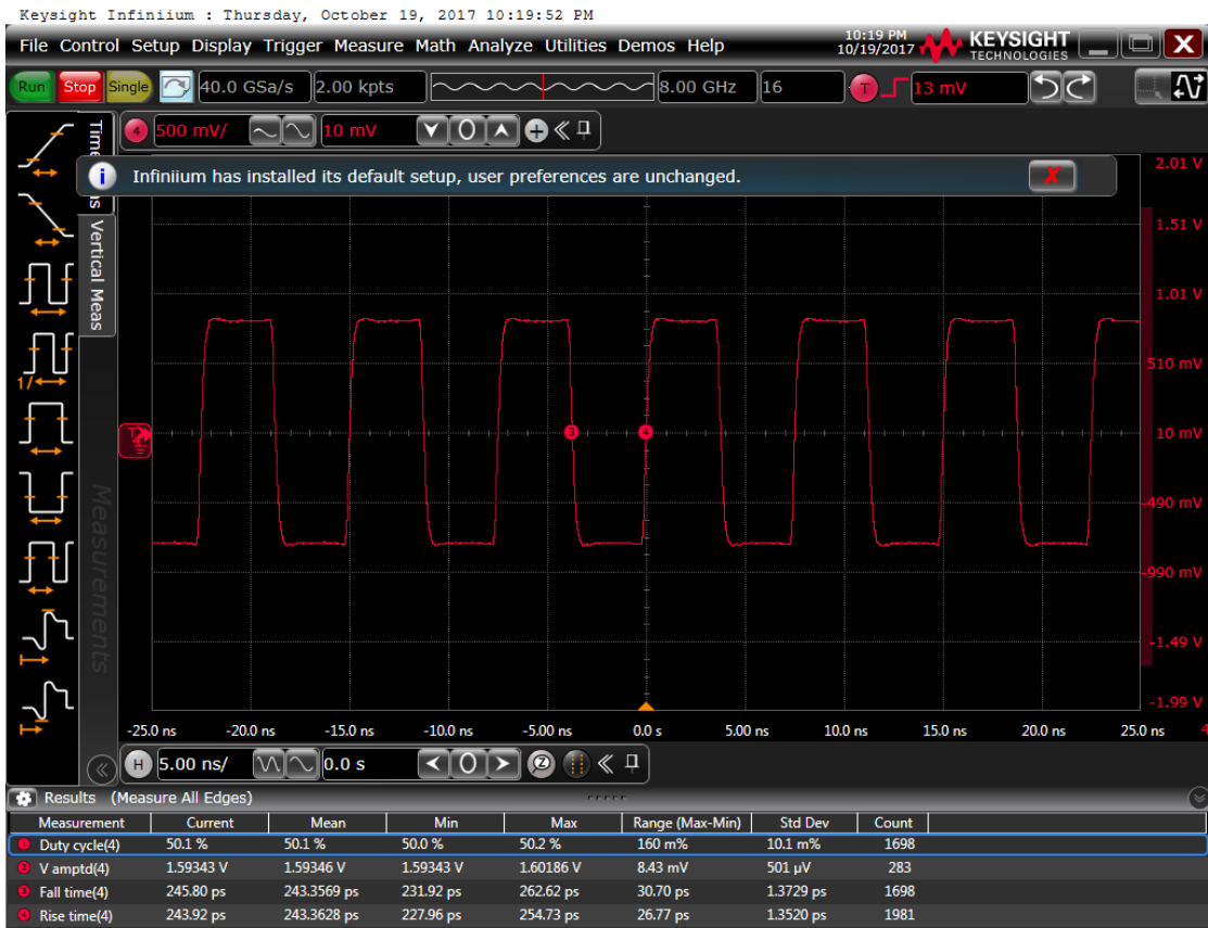
Figure 7: Output waveform, 3.3 V
