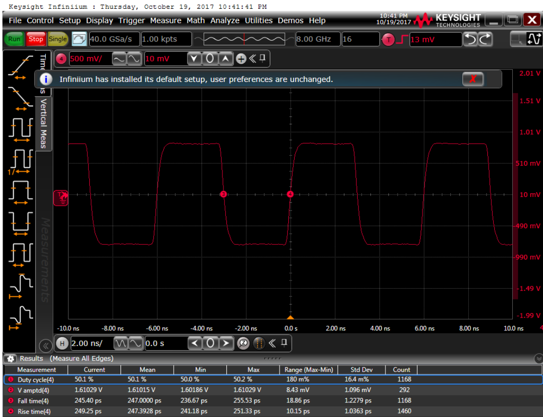
Figure 7: Output waveform, 3.3 V
