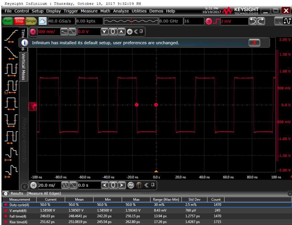
Figure 6: Output waveform, 2.5 V
