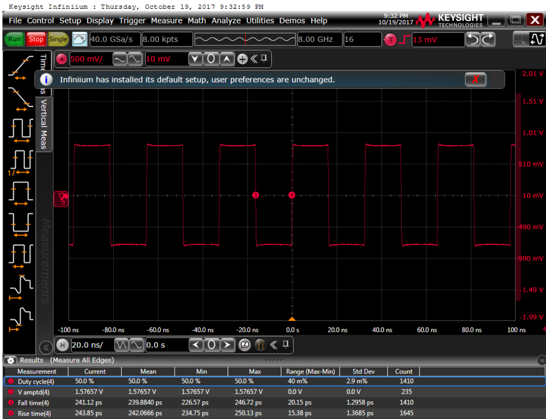
Figure 7: Output waveform, 3.3 V
