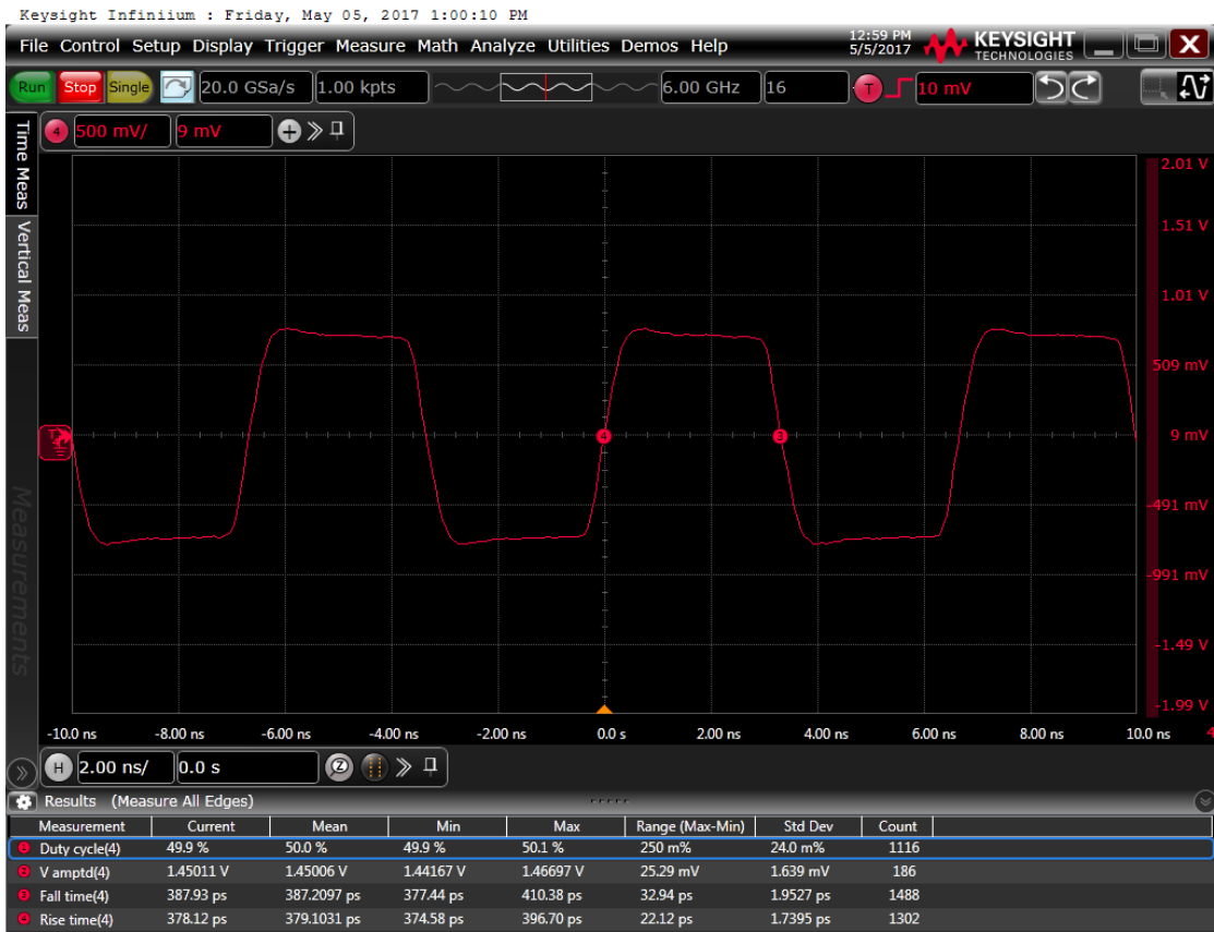
Figure 6: Output waveform, 2.5 V
