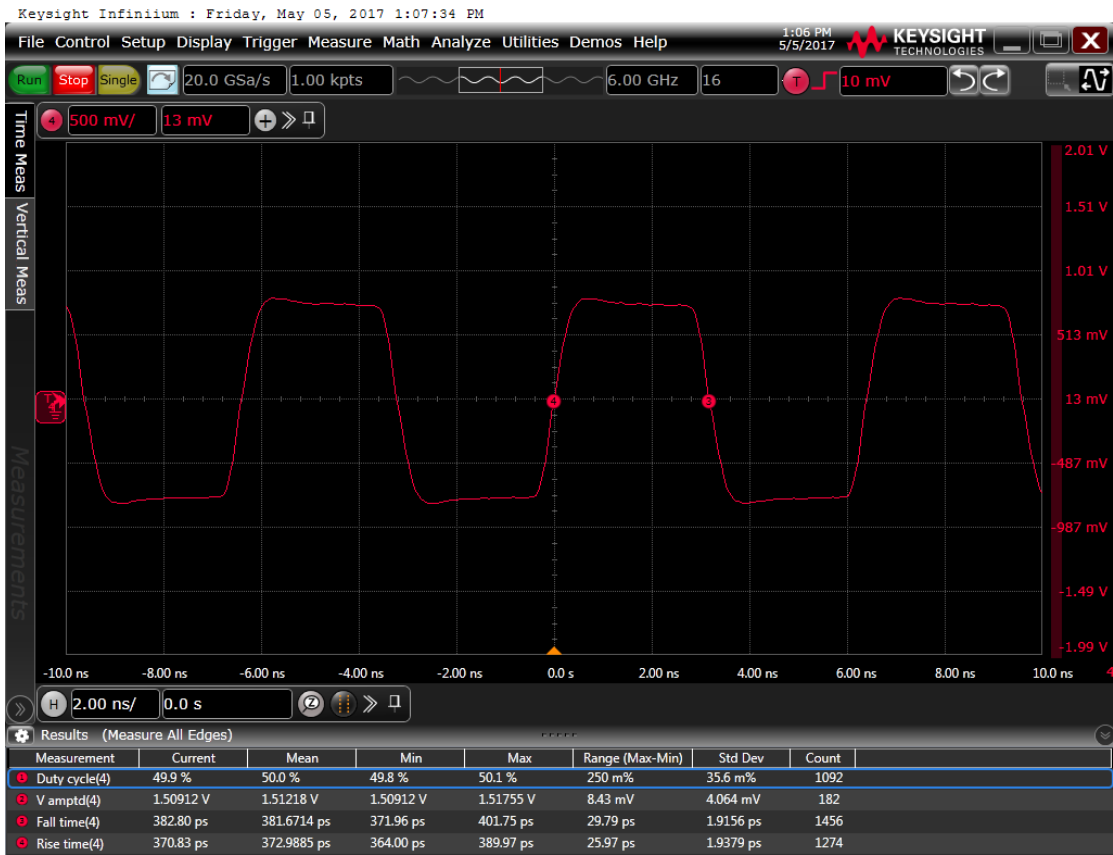
Figure 7: Output waveform, 3.3 V
