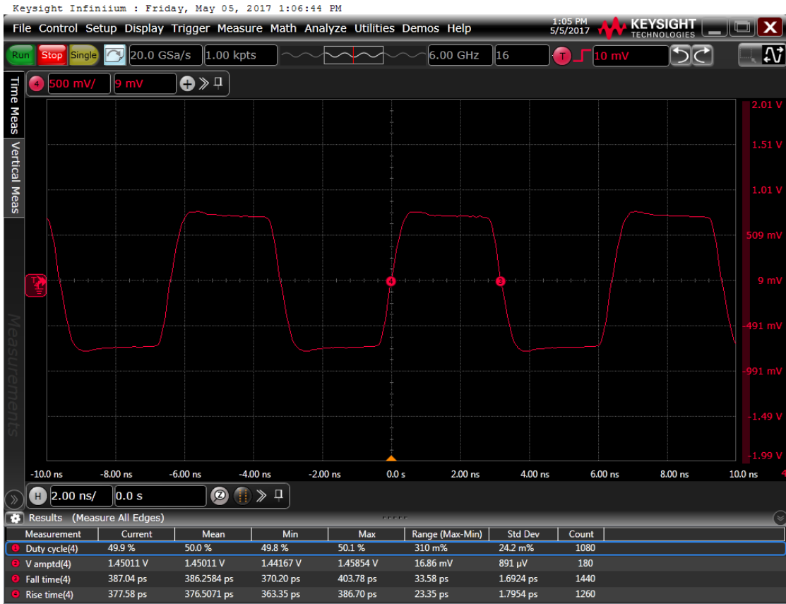
Figure 6: Output waveform, 2.5 V
