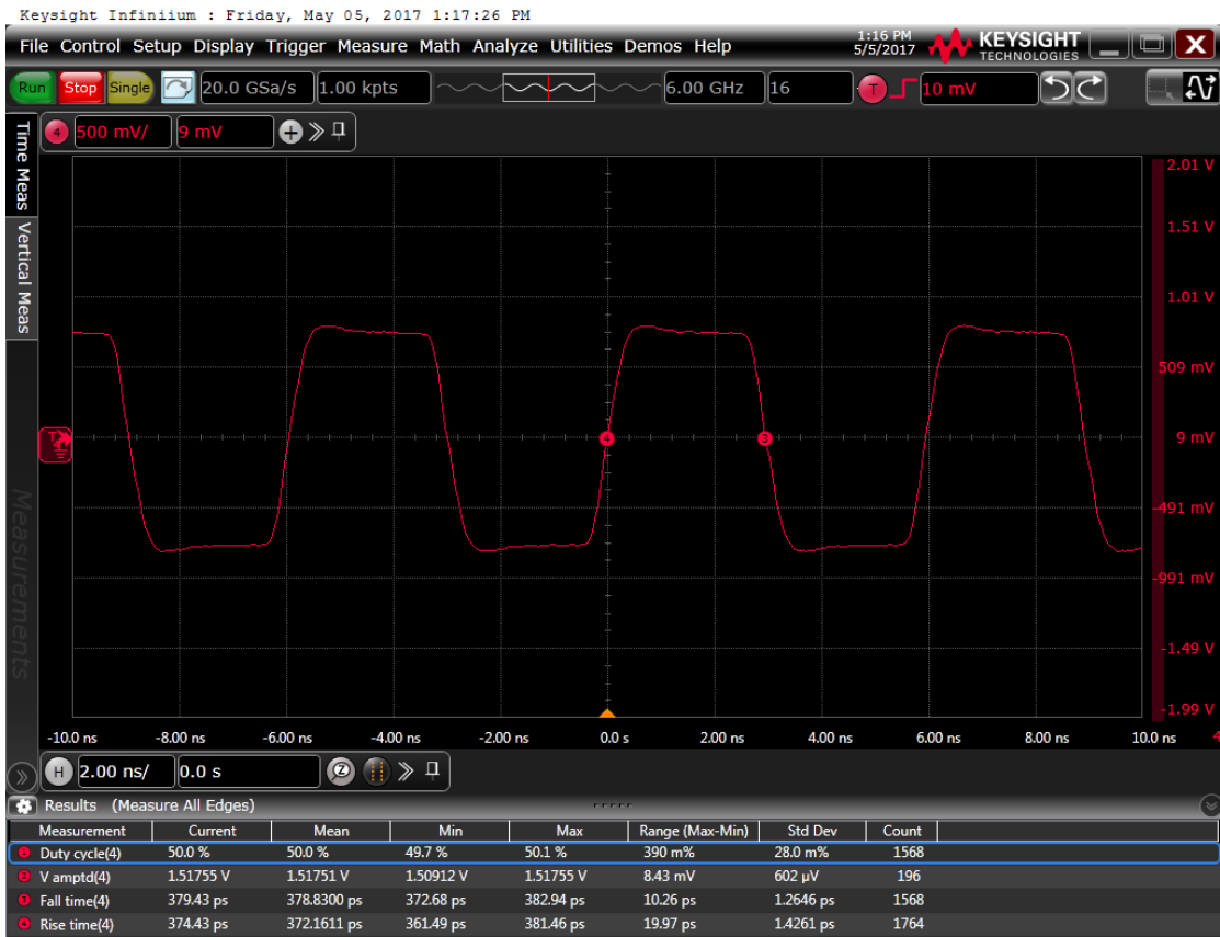
Figure 7: Output waveform, 3.3 V
