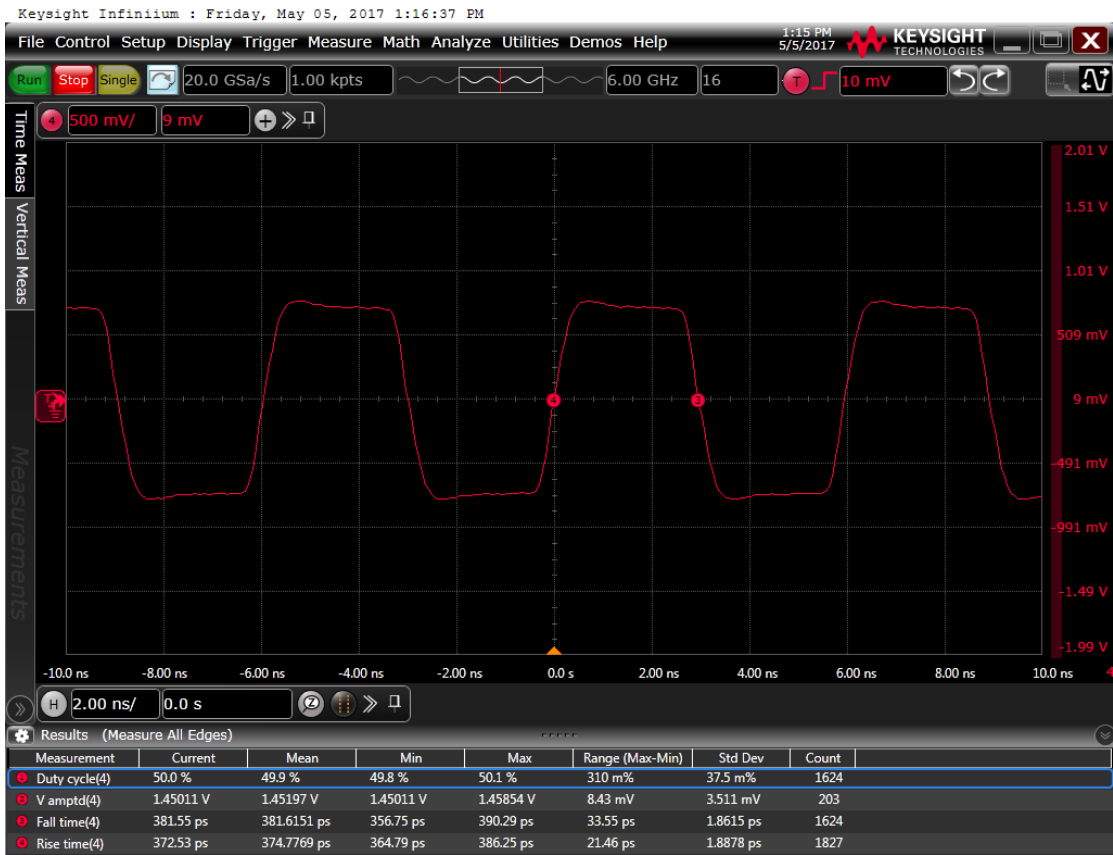
Figure 6: Output waveform, 2.5 V
