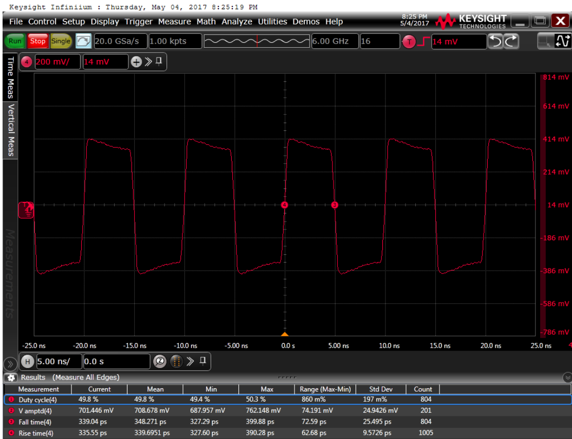
Figure 7: Output waveform, 3.3 V
