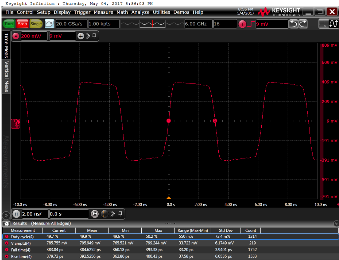
Figure 6: Output waveform, 2.5 V
