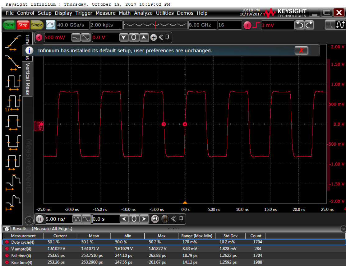
Figure 6: Output waveform, 2.5 V
