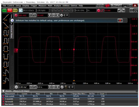
Figure 6: Output waveform, 2.5 V
