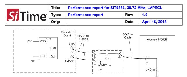
Figure 3: Test setup for measuring phase noise.
