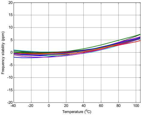
Figure 9: Frequency stability over temperature, 3.3 V
