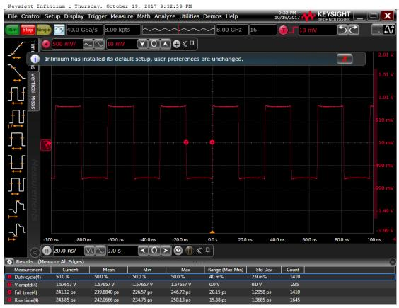
Figure 7: Output waveform, 3.3 V
