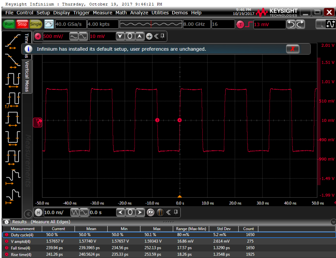
Figure 7: Output waveform, 3.3 V
