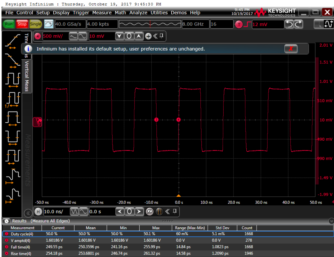
Figure 6: Output waveform, 2.5 V
