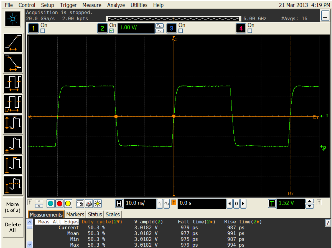
Figure 4. Duty cycle, Rise/Fall time and Amplitude 3.0V
