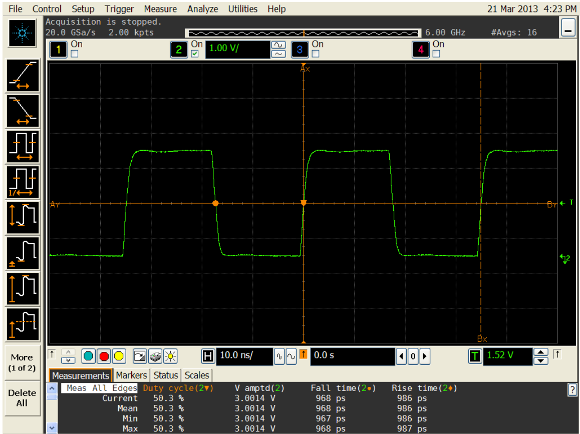
Figure 4. Duty cycle, Rise/Fall time and Amplitude 3.0V
