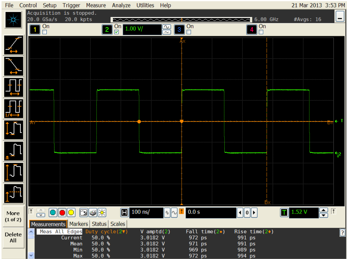
Figure 4. Duty cycle, Rise/Fall time and Amplitude 3.0V
