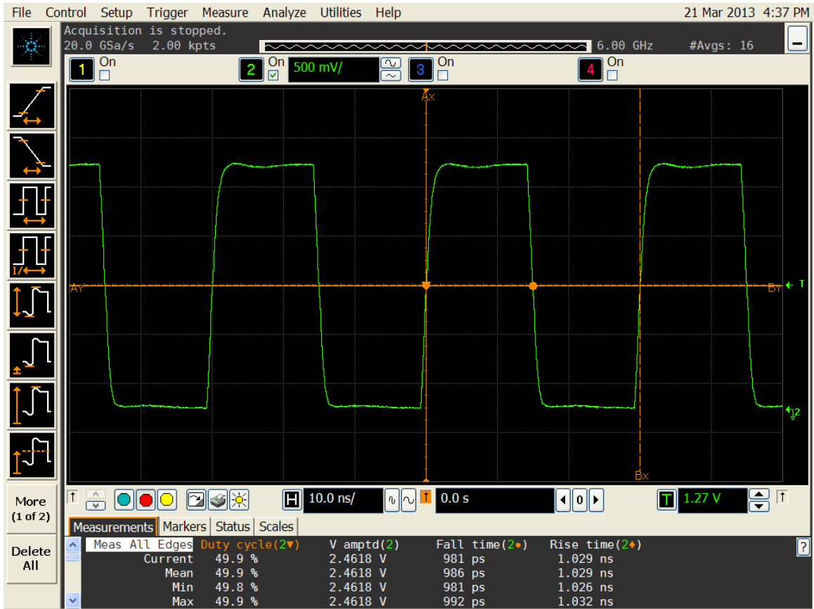
Figure 2. Duty cycle, Rise/Fall time and Amplitude 2.5V
